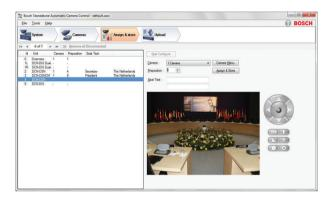
DCN-SWSACC Standalone Automatic Camera Control of the DCN Conference systems interfaces with the Bosch Allegiant or Autodome. It selects fixed or movable cameras to be activated to display the current active speaker at a conference.
