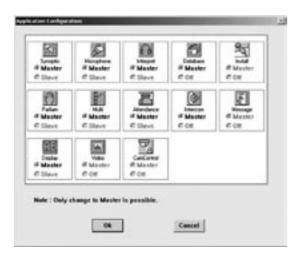
The Multi PC software module is needed when more than one PC is required to control the DCN Next Generation system. All Slave PCs in a multi-PC environment are connected via Ethernet to the Master PC, which is connected the CCU.
