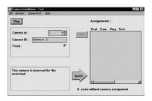
The DCN Next Generation Automatic Camera Control software interfaces DCN Next Generation congress systems with the Bosch Allegiant series of video control switchers. It selects fixed or pre-positioned cameras (such as the Bosch AutoDomes) to be activated to display the current active speaker at a conference.
